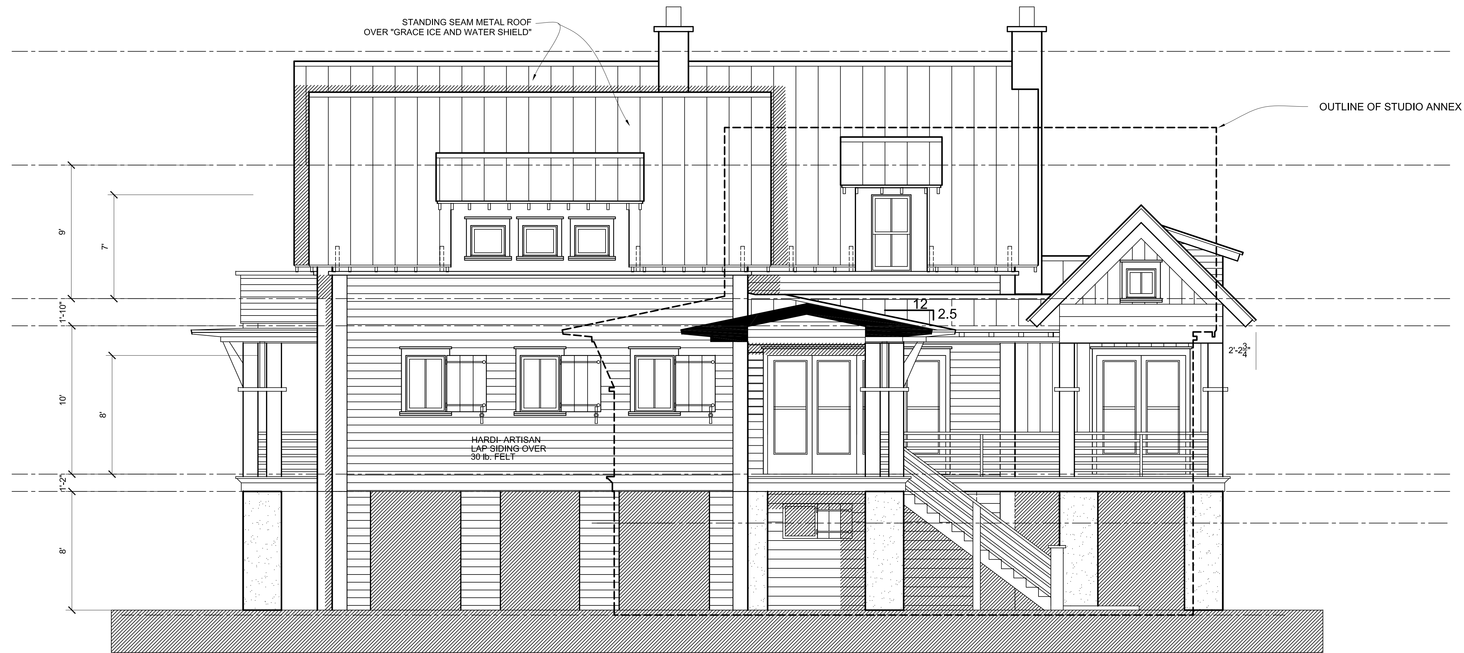
rear elevation - shown without annex 1/4" = 1'-0"
